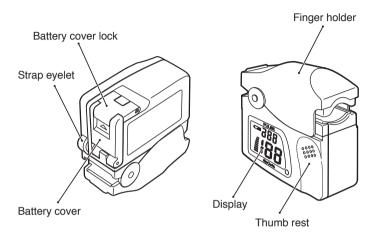
Battery cover: Open or close this cover when replacing the
